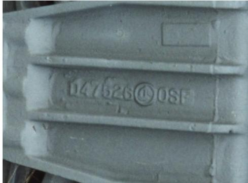
It is not uncommon for a company, when pressed to complete orders, to subcontract some of their work to another company in order to deliver on schedule. This appears to be the inclusion of both companies' symbols for to be placed on the part for traceability.
